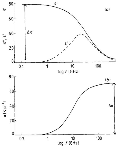
**Figure 2.** The dielectric dispersion exhibited by pure water at 20 °C, illustrated in terms of the change in (a) the real ( $\epsilon'$ ) and imaginary ( $\epsilon''$ ; dielectric loss) parts of the permittivity and (b) the frequency dependence of the conductivity. The low-frequency conductivity at neutral pH, due to the presence of  $H^+$  and  $OH^-$  ions, has a value of some  $5 \mu S m^{-1}$ .
