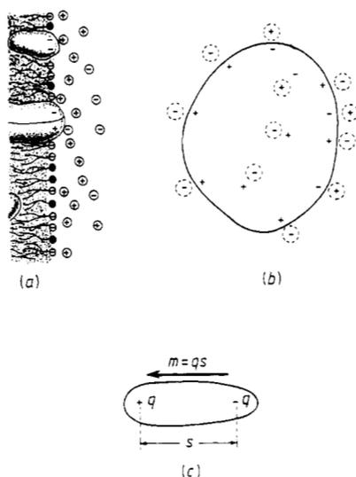
**Figure 1.** An illustration of the electrical double layers formed at the surface of a charged biological membrane (a) and around a charged, aqueous globular protein (b). (c) A simple polar molecule, consisting in this case of a pair of opposite unit charges  $+q$  and  $-q$  separated by a distance  $s$  and possessing a dipole moment of  $m = qs$  C m.
