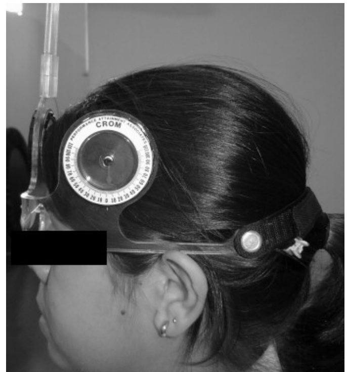
Figure 2. Side view of correctly positioned cervical range of motion instrument (CROM).
