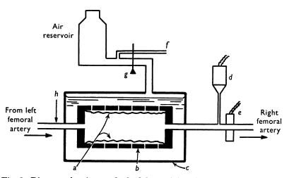
Fig. 1. Diagram showing method of determining the pressure-flow curve of the femoral vascular bed. a, condom rubber sleeve; b, perforated Perspex tube; c, Perspex chamber; d, Statham strain-gauge manometer; e, blood flow probe; f, air-leak by-pass; g, position of clamp on two tubes; h, position of clamp on femoral arterial tubing. The horizontal arrows indicate the direction of blood flow. For details see text.
