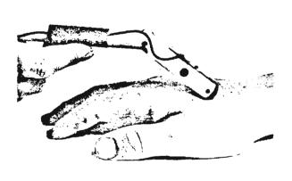
FIGURE 1 Meridian scanning probe: the teflon body is constructed in two parts with a flexible joint between the two and a metal insert to furnish weight in the distal portion. The electrode proper is a stainless steel wheel on a stainless steel spindle with low friction between it and the teflon. This probe design permits constant pressure and no drag between the skin and the wheel contact.
