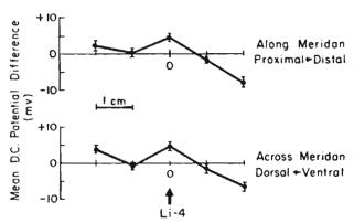
FIGURE 7 Direct current potentials measured along the meridian (top trace) and at right angles to the meridian (bottom trace) at point Li4. The point itself is significantly more positive than the remainder of the trace.
